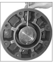
Fig. 4.12 Tightening Retainer Set Screw
