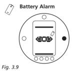
The battery alarm icon, Fig. 3.9, is displayed when the actuator detects its battery as being low, discharged or missing.
