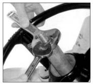
Fig. 5.6 Down Stop two Spanners
