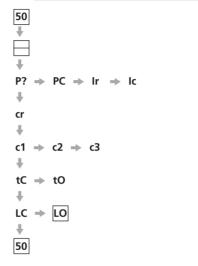
**NOTE:** When in checking mode Set Limit Open **[LO]** does not appear.
