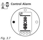
The control system alarm icon, Fig 4.5, is displayed when the remote control system maintains an active ESD or interlock signal (the ESD, interlock function or conditional control having been enabled.) Local and Remote operation will be inhibited while an active ESD or interlock signal is present (refer to [A1] ESD Action page 34, [A8] External Interlocks page 36 and Conditional Control [A9] page 36.)
