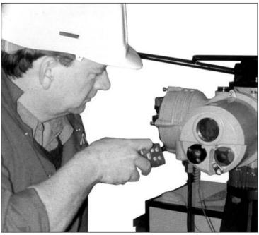
The actuator's Primary Function settings affect the correct operation of the valve by the actuator. If the actuator has been supplied with the valve, the valve maker or supplier may have already made these settings.
